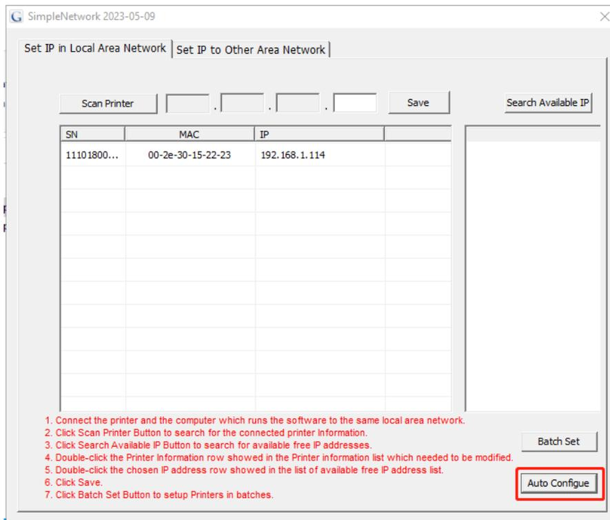
6. Click "Scan Printer", a new IP address will be appeared, it is the IP address under the current network segment.
